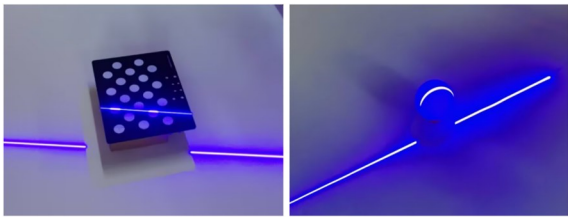
(a) 标定板重建 (b) 标准球重建 (a) Calibration plate reconstruction (b) Standard ball reconstruction
