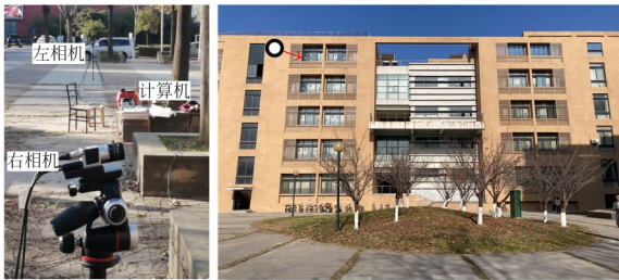
图 16 室外双目相机标定实验 Fig. 16 Experimental setup for outdoor stereo camera calibration
