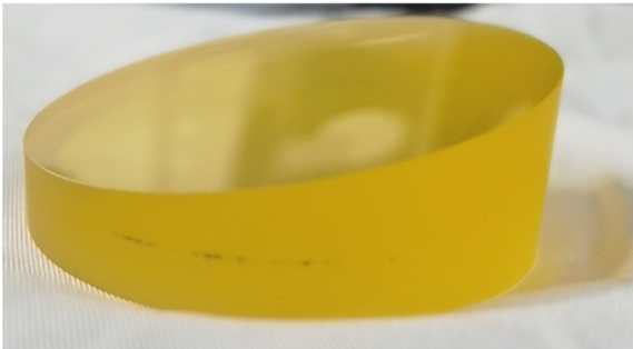
图8 离轴量为 35 mm、尺寸为 50 mm 的离轴抛物镜 Fig. 8 Off-axis parabolic mirror with an off-axis distance of 35 mm and a size of 50 mm
