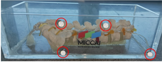
图 3 器械 2(红圈处为光学标记点) Fig. 3 Instrument 2(The red-circled region indicates the optical marker)
