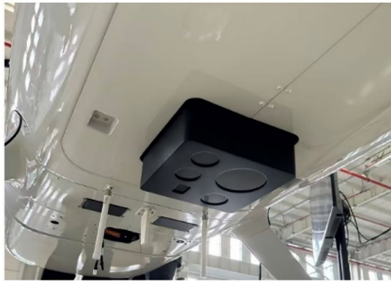
(c) 光学吊舱安装在复合翼无人机上 (c) Optical pod mounted on UAV
