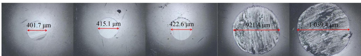
(b) 不同沟槽深度(10~50 \mu\text{m} )条件下ZrO 2 陶瓷球的磨斑图像 (b) Wear scar images of ZrO 2 ceramic balls under different groove depths (10~50 \mu\text{m} )
