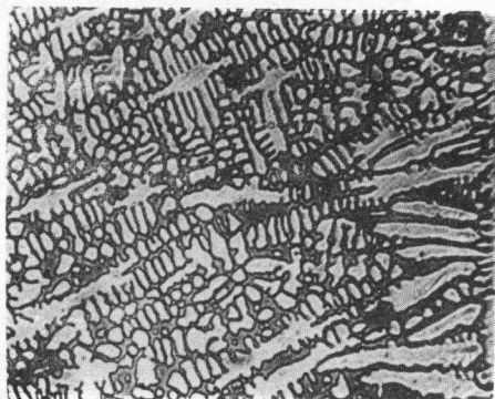
Fig. 7 The microstructure of cross-section of Ni 01 alloy layer 500×
