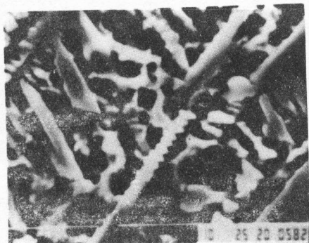
Fig. 5 The morphology of phase CrB in Ni 03 alloy layer, SEM
