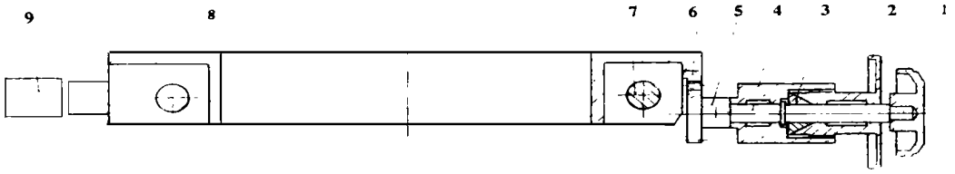
1. hand wheel for scanning 2. hand wheel for locking 3. lock ring 4. axle 5. gear 6. rack 7. guid rod 8. slide plate 9. grating scale
