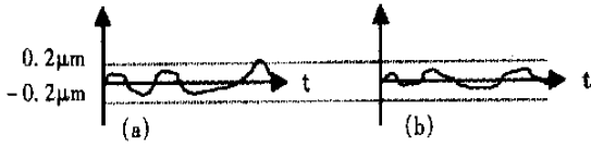
Fig. 5 The influence of laser power on focus
