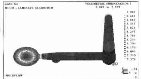
Fig. 8 Volumetric shrinkage after holding process
