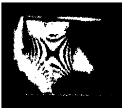
Fig. 3 Interferogram of optical testing using VLS flat grating
