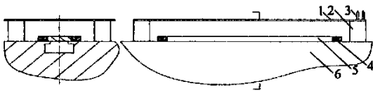
1. Heater 2. Heat - insulating support 3. Junction box of transformer 4. Heat- insulating plate 5. Simulating part of machine bed 6. Table of milling machine
