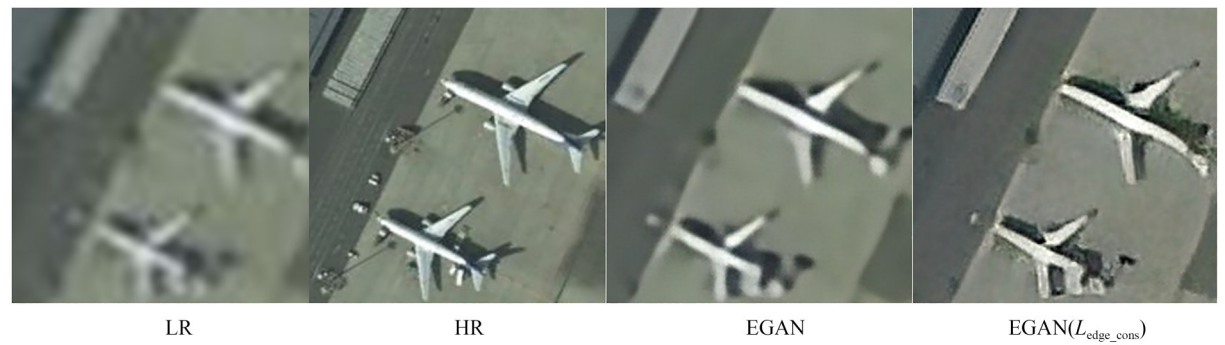
图 7 引入边缘一致性损失 L_{\text{edge\_cons}} 对比图 Fig. 7 Comparison of L_{\text{edge\_cons}} with edge consistency loss
